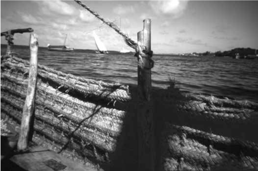
Matting woven from zikoma (palmetto) fronds lashed to the sides of the dhow with kamba (rope) made from coconut-husk coir.
